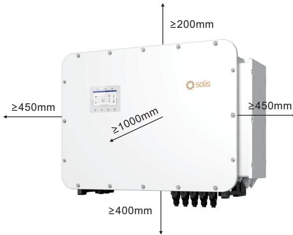
Figure 3.5 Inverter Mounting Clearances
