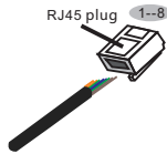
Figure 3.39 Strip the insulation layer and connect to RJ45 plug
