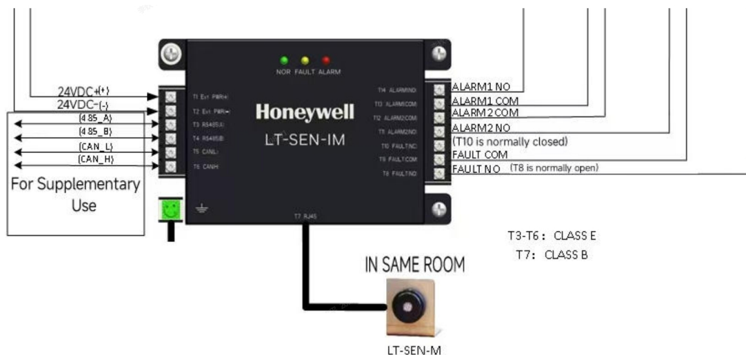
Figure 7-4 Flammable gas detector wiring diagram
